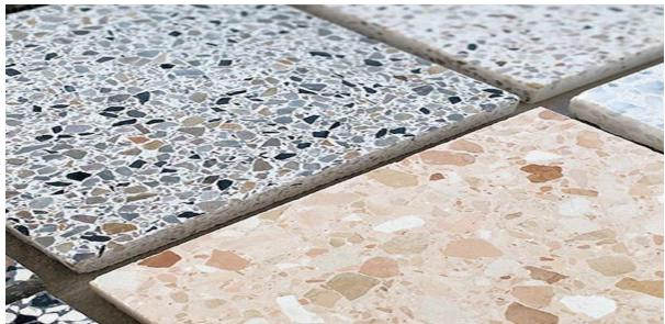
This floodproofing method involves using materials that reduce flood damage and speeds post-flood clean up. Such materials include non-paper-faced gypsum board and terrazzo tile flooring and can also include the use of floodproof cabinets and the replacement of wooden doors.
