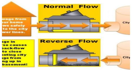
Designed to keep raw sewage out of your home in the event of sewer overflow. A backwater valve connects to your home's plumbing and features an internal mechanism called the "flapper." In the event of sewer overflow, the flapper closes to help protect your home from filling with raw sewage.
