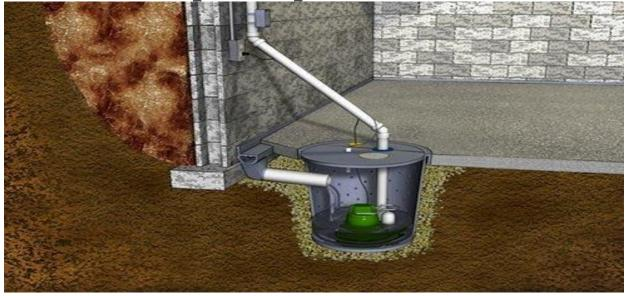
A sump pump is a small pump installed in the lowest part of your basement. Its purpose is to collect subsurface water from the ground near your home's foundation and pump it out to your yard to keep your basement dry.
