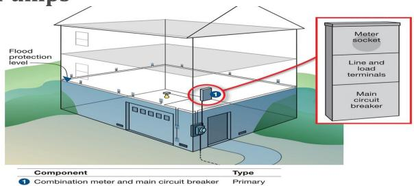
Relocating mechanical equipment above the flood elevation or out of your basement could significantly reduce the risk of critical systems being damaged during a flood. Raising mechanicals will not significantly reduce flood insurance premiums. Installing a heat pump is an eligible flood mitigation activity.
